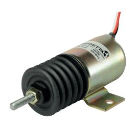
The P610 range of solenoid actuators are a dual wound design with independent control coils for both pull and hold functions. The advantage of separately controlled coils is that, when wired correctly, there is less risk of pull-in coil burnout as there is with dependently switched modules. The P610 range offers high pulling power in a compact package. Ideal for a vast range of applications in both stationary and mobile plant and equipment.
